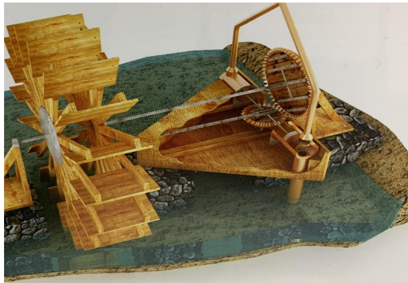
Figure 3. water-raising machine (include Piston, cylinder, valve) ([6])
