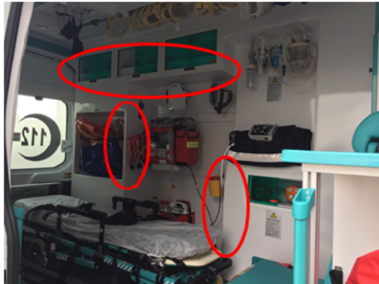
Figure 2: Sharp corners in the cabin.
