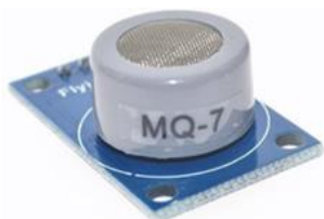
Figure 1. The picture of a semi conductive metal oxide CO sensor with MQ-7 brand.
