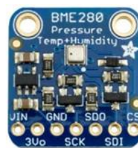
Figure 2. The picture of a BME280 branded pressure-temperature-humidity sensor.
