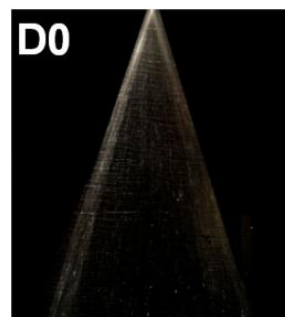
Figure 10. Flow visualization for the baseline D0 design showing the sweep angle of the oscillating jet generated by the oscillator.
