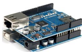
Figure 3. The picture of microprocessor (bottom component) and Ethernet shield (top component) together.
