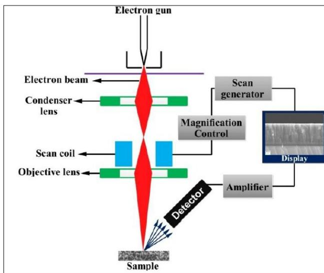
**Figure 1.** A schematic diagram of SEM (Raza, 2012)
