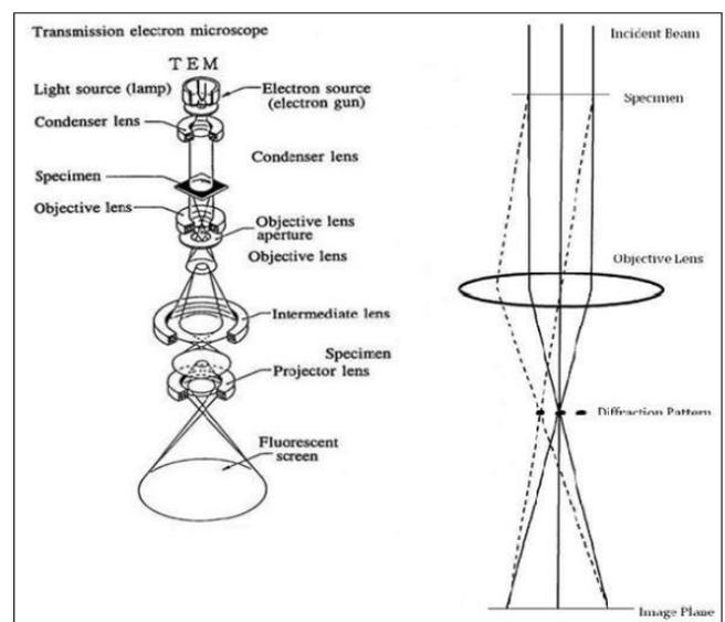
**Figure 2.** The layout of optical components in a basic TEM (Williams and Carter, 2009).
