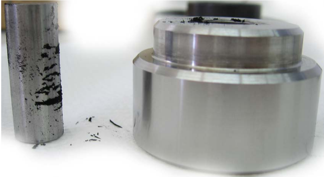
Figure 3: The Mold which Ppy was Placed in, before Applying Pressure.
