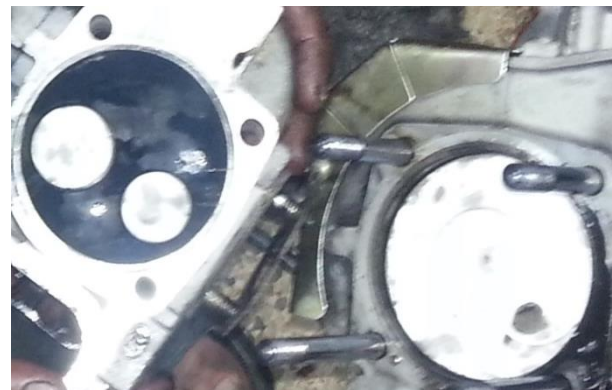
Figure 2. Pistons and valves coated by APS
