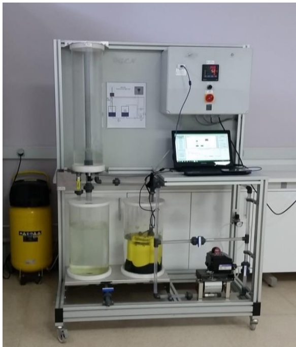
Figure 2. Experimental system: on-line computer connected to the liquid level control system
