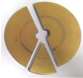
Figure 2. Example of disc cut to measure thickness.
