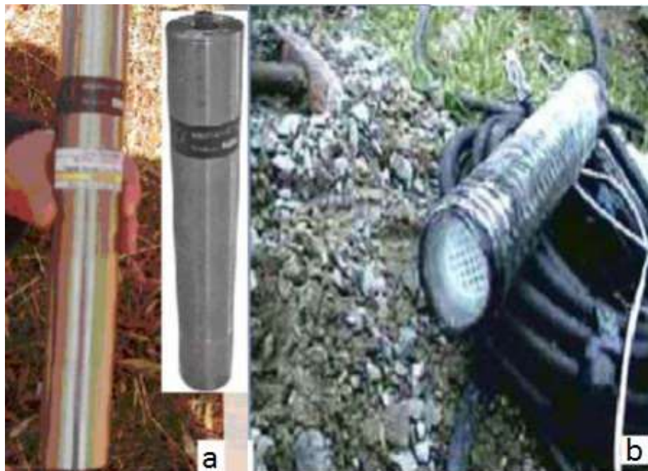
Figure 3. (a) Alphaspector 611 model, (b) Prepared to bury the Alphaspector probe.
