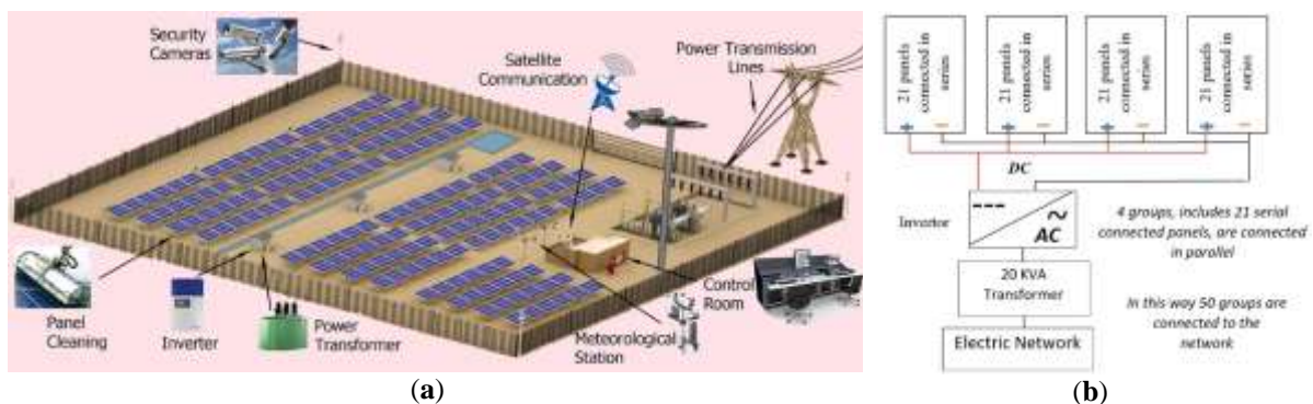
Figure 1. (a) Representative view of solar power plant in Konya region. (b) Solar power plant single line scheme.
