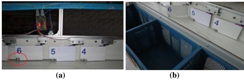
Figure 2. Installation of baffle gates (a), operation of baffle gates (b) (Ornek, 2014).
