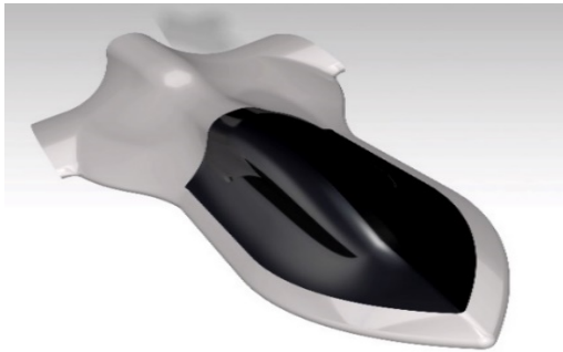
Figure 8. Model 4 nose form, battery compartment design. The black and grey sections represent the sliding cover and the fixed section, respectively.
