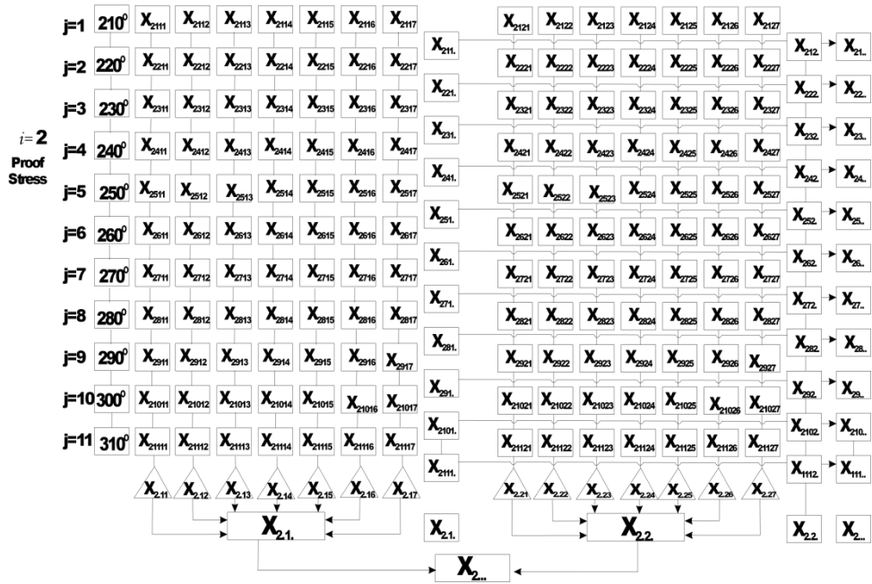
Figure 2. Split-split plot Analytical Design of the Effect of Barrel Temperature on Proof Stress.
