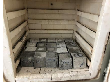
Figure 1 Interior of a High Temperature Oven
