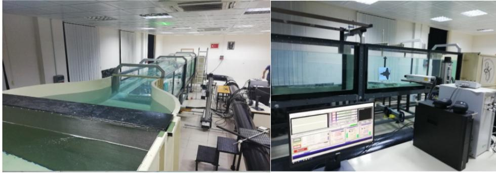
**Figure 2:** The closed-loop, open water channel experiment setup
