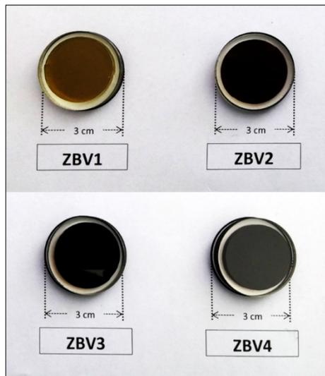
**Figure 1:** Synthesized ZnO-B<sub>2</sub>O<sub>3</sub>-V<sub>2</sub>O<sub>5</sub> glass samples
