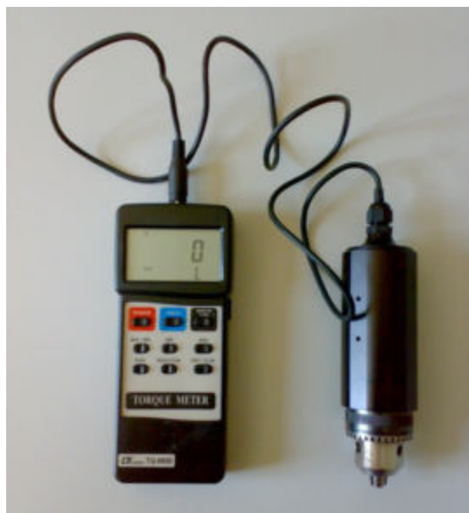
Fig. 2. Photograph shows the torque-meter device
