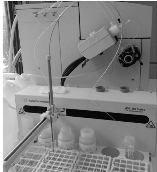
**Figure 1.** ICP-MS device
