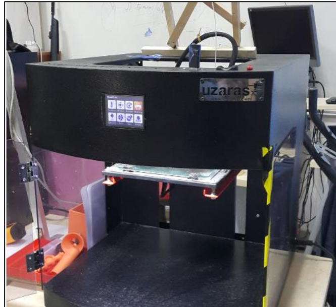
Figure 1. Dream maker 3D printer where tensile and bending samples are produced
