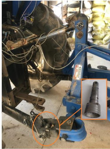
Figure 3. Force-measuring pins to measure the draft forces
