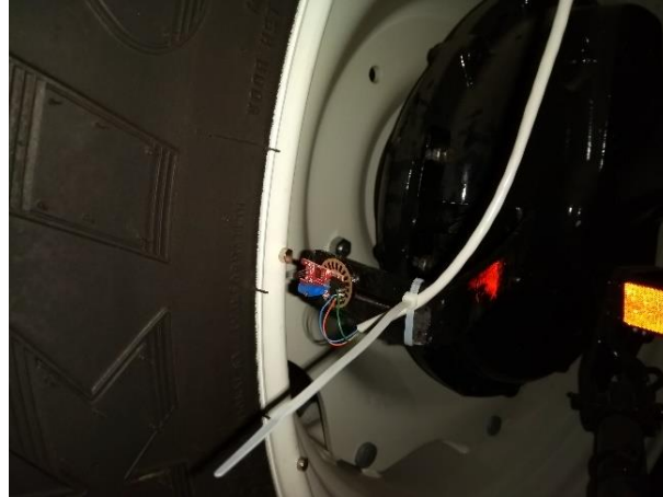
Figure 1. Hall effect sensors and neodymium magnets
