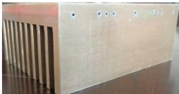
Figure 2. The photo of the aluminum fin block heat sink and the thermocouple holes
