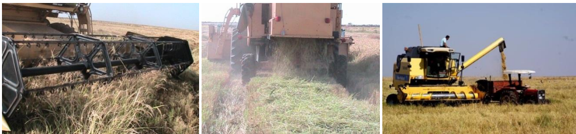
Figure 3. Directly paddy harvesting by self-propelled combine- harvester.
