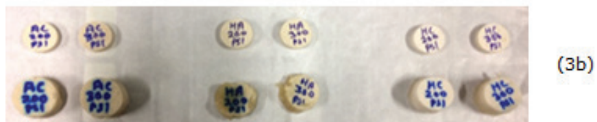
Figure 3. Swelling behaviour of tablets (3a); Camera image before and after swelling (3b).
