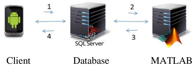
Figure 2. The general structure of mobile diagnosis system
