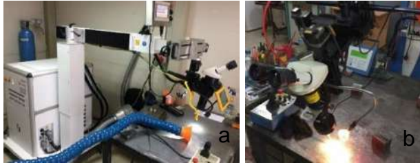
Figure 1. a) Pulsed fiber laser welding machine (Alseko-Sisma SWA 300) b) TIG welding machine (Tig-400) c) Ti-6Al-4V sheet technical drawing.
