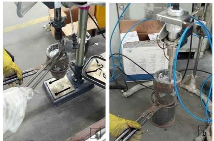
Figure 2. (a) Mechanical stirring, (b) ultrasonic vibration
