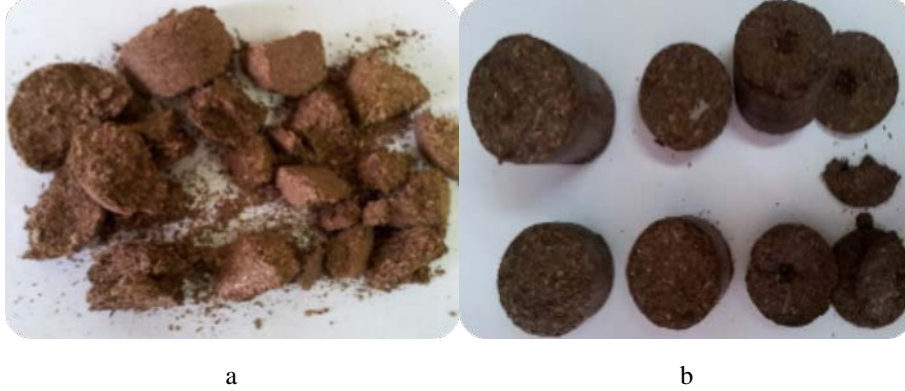
Figure 4. Hazelnut husk briquettes after Tumbler testing (a: T1, b: T7)
