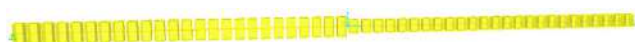
Figure 2 FE model for simply supported stepped beam on elastic foundation (50 beam elements)
