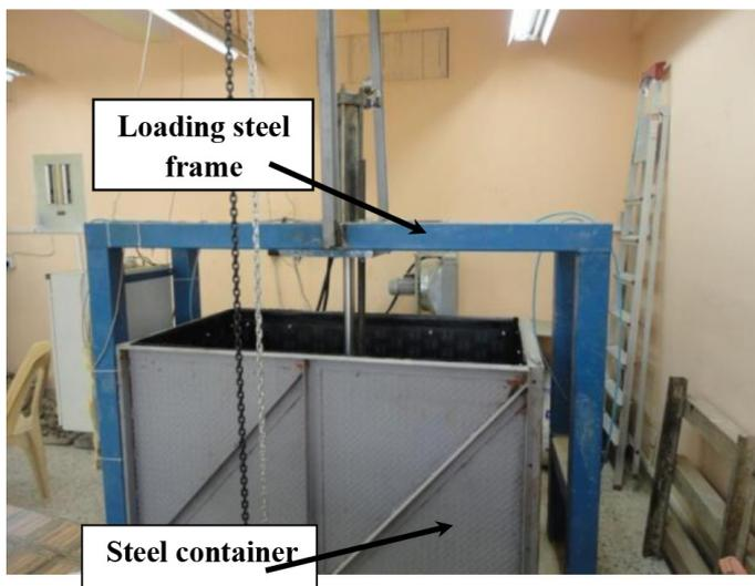
Figure 4. Steel frame of the loading system.
