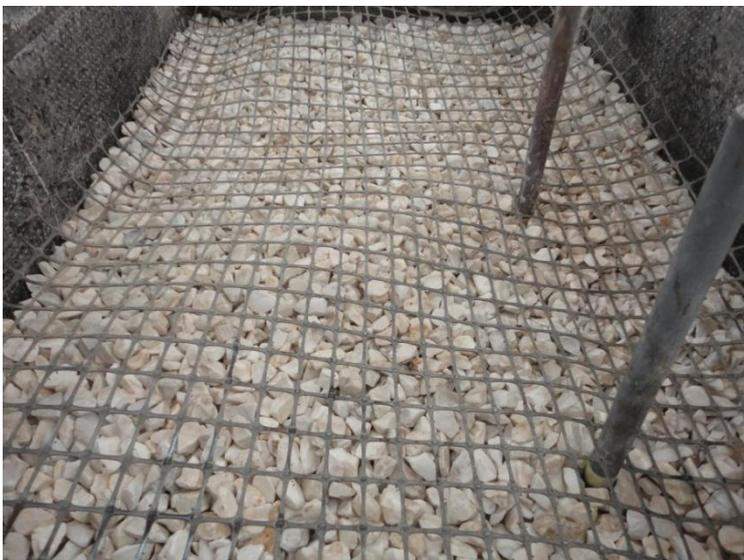
Figure 10. Placing the geogrid.
