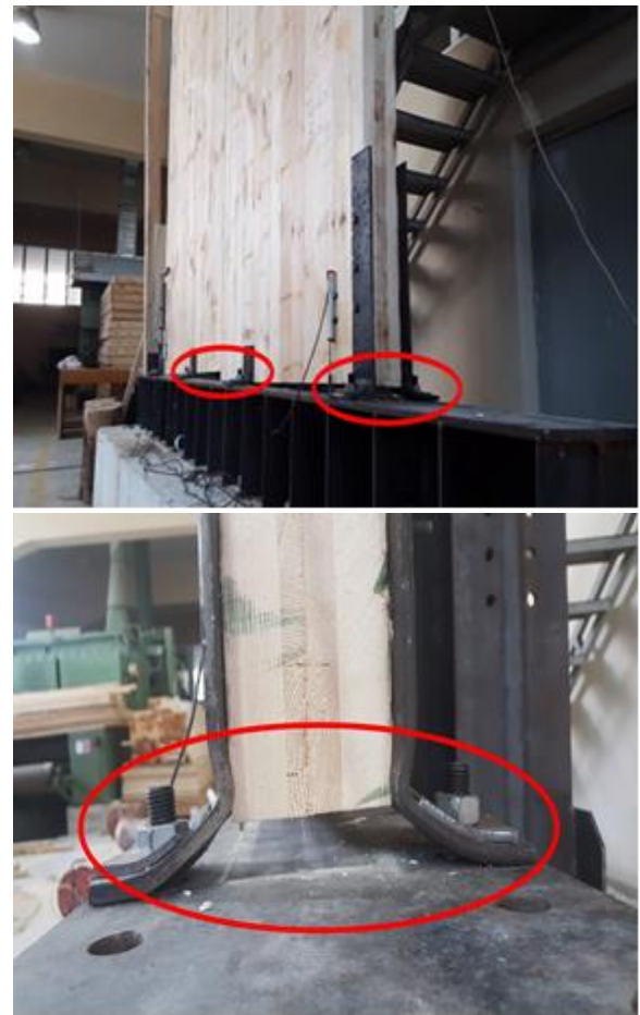
Figure 6. Failure modes of CLT shear walls.
