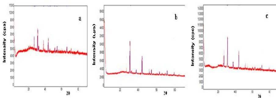
FIGURE 6. X-ray powder diffraction patterns of sample (a) Co-1, (b) Co-2, (c) Co-3.
