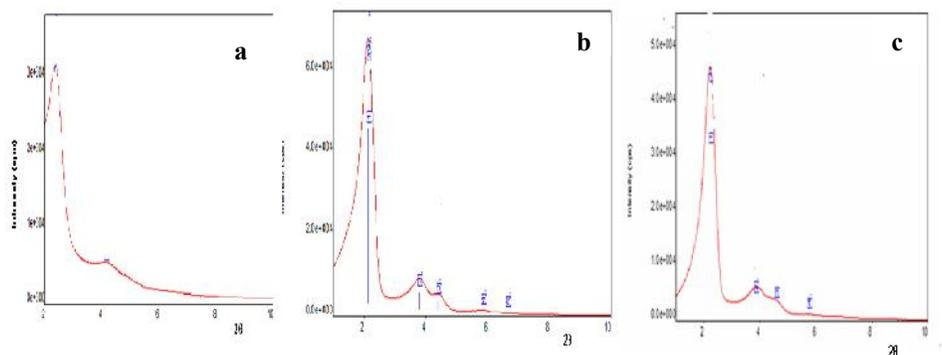
FIGURE 1. X-ray powder diffraction patterns of sample H-1 for different calcination temperatures (a) 450°C, (b) 550°C, (c) 650°C.
