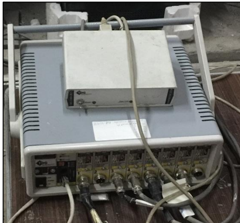
Figure 4. Signal conditioning and data acquisition system (SCDAS)
