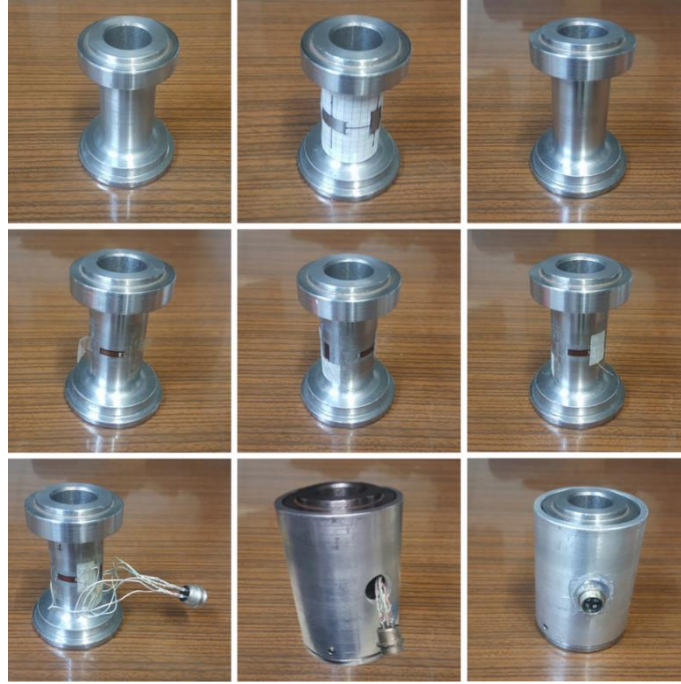
Figure 3. Load cell production steps
