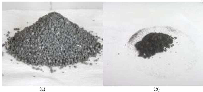
Şekil 2. Stabilize ve kurutulmuş arıtma çamuru (a) ve elde edilen humik asit (b) Figure 2. Stabilized and dried sewage sludge (a) and obtained humic acid (b).
