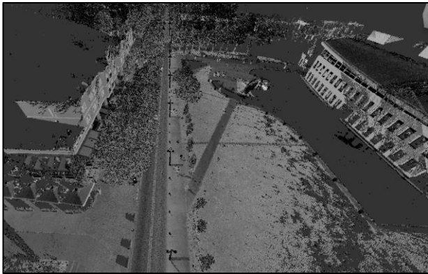
Figure 3. ITU Ayazaga Campus Scanning by Riegl VMX 450 MLS
