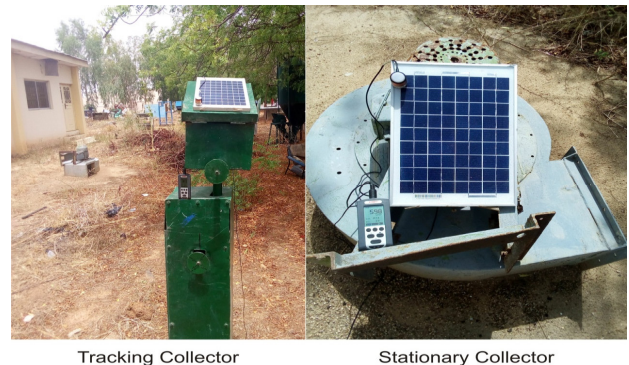
Figure 3. Experimental Set-up showing tracking collector and stationary collector
