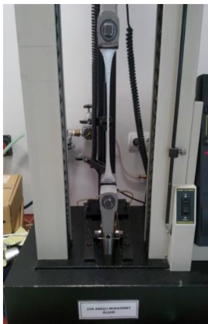
Figure 2. Elongation of aluminized aramid fabric
