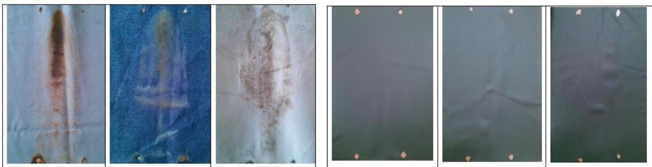
Figure 4. 350g - molten aluminium tested samples and related PVC skin simulat (from left to right: LenzingFR-Wool-Polyamide, Cotton 3-Denim, leather)
