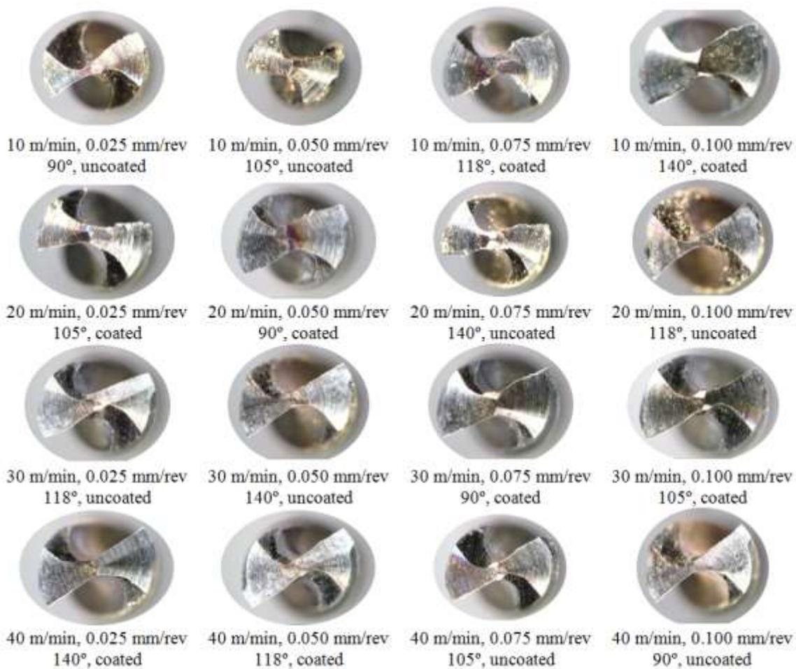
Figure 4. Used drill bit in experiments
