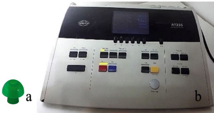
Figure 2. 13 mm mushroom shaped rubber probe tips (a) and audiometry device (Interacoustics AT235h®, Denmark) (b).
