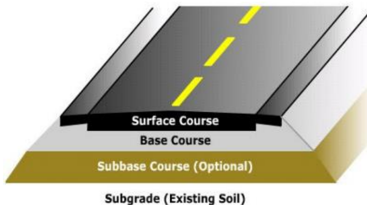
Figure 3. A typical flexible pavement section view [23]
