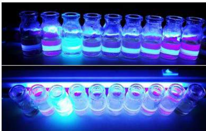
Figure 3. Photograph of the fluorometric responses of sensor V toward various anions in THF-H 2 O (70:30, v/v)
