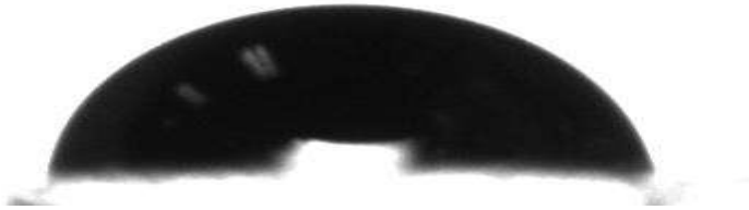
Figure 3.1. Contact Angle Image of Uncoated Glass
