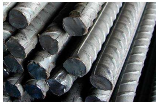
Fig. 2. A view of steel rebar tips with ribs
