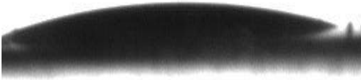
Figure 3.2. Contact Angle Image of TiO_2 Coated Glass
