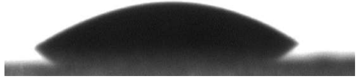
Figure 3.3. Contact Angle Image of Boron Oxide Coated Glass
