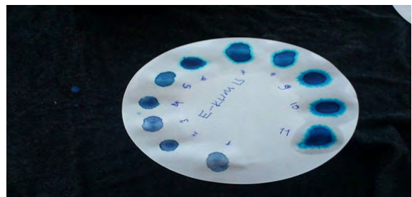
Figure 2. Determining the methylene blue value of sand
