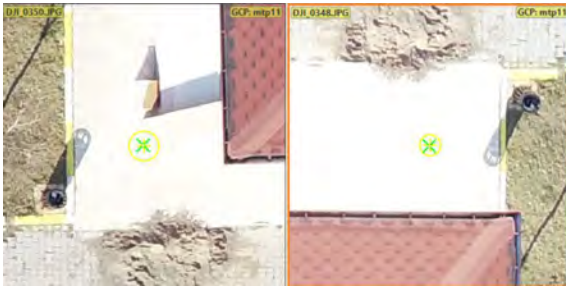
Figure 12. Challenges acquiring data from photogrammetric model. At C12, color of the building over-radiated at the time of photoshoot and may lead to a poor positioning assessment. Green cross represents the estimated location and yellow circle is the error estimation for the point.
