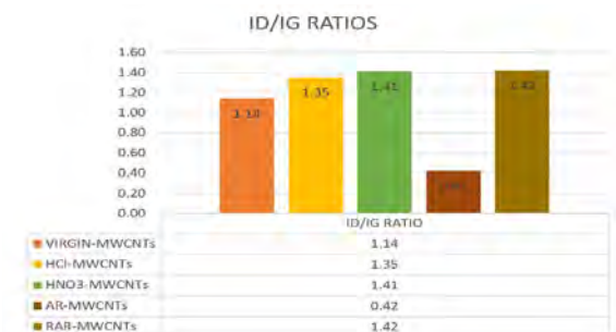
Figure 4. ID/IG ratios obtained from the analysis of Raman spectra.
