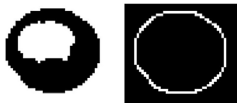
Figure 2. a) Binary image of a bubble b) bubble edge obtained with MATLAB code.
