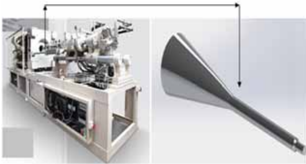
Figure 1. Ekin 160 – B plastic injection machine and its injection nozzle
