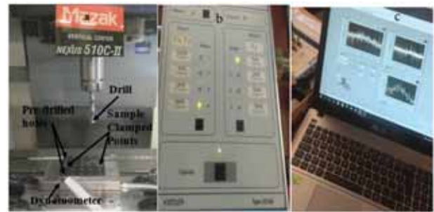
Figure 1. Experimental Setup (a) MAZAK Vertical Centre NEXUS 510 C-II Model Milling Machine and Dynamometer Apparatus, (b) Kistler Type 5233 A Model Data Logger, (c) Computer.
