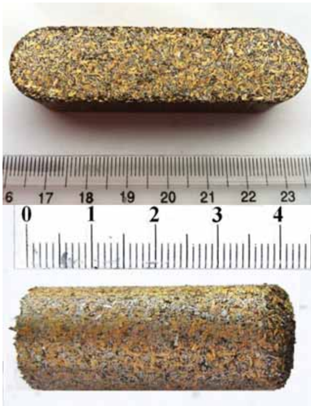
Figure 1. Cold pressed specimens: (a) prismatic and (b) cylindrical
