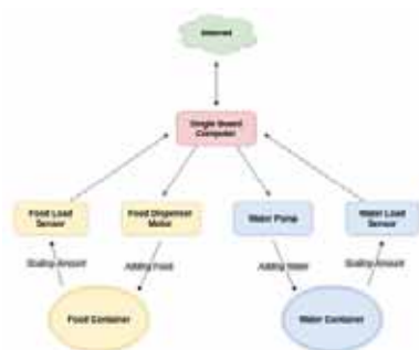
Figure 2. Performing Unit components and flow diagram of the designed IoT.
