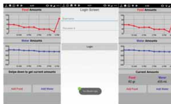
Figure 5. Mobile Application main screens. The graphs are for monitoring the current amounts of food and water over a pre-defined time period
