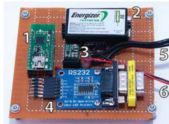
Figure 3. Electronic circuit built for interface, transmission and power. Photograph of the electronics transmitter. 1: Modified Wixel board. 2: battery. 3: step-down converter. 4: UART-RS232 board. 5: power supply to acoustic modem. 6: power supply connector to battery
