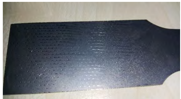
Figure 4. b) Clamping marks, slippage observed.
