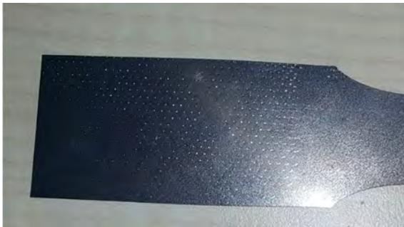
Figure 4. a) Clamping marks, no slippage observed.
