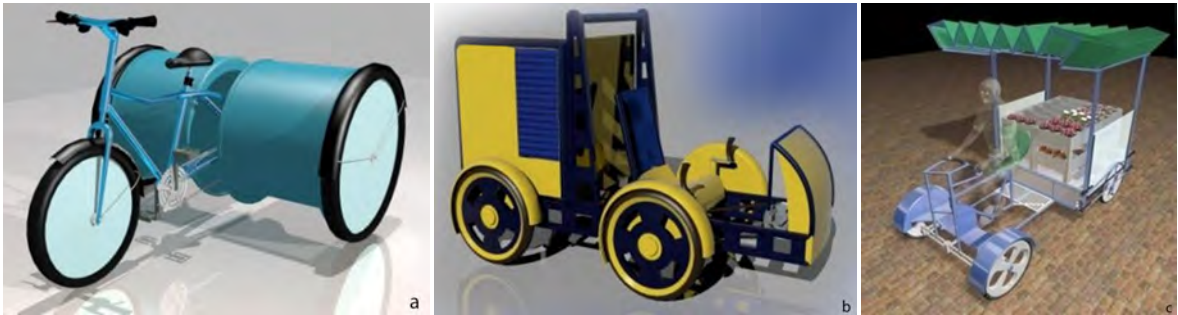
Figure 6. a) Tricycle to carry water demijohns, b) A manpowered vehicle to carry mail, c) Manpowered vehicle to sell flowers
