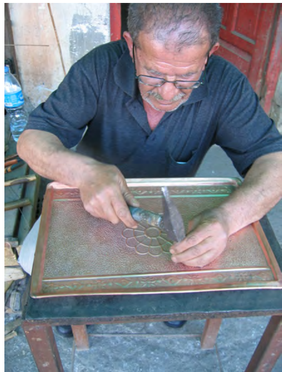
Figure 5. Forming the copper tray with embossing method; the tray is completely made with traditional method. Design S.Satir, Production: Zülfikar Usta.
