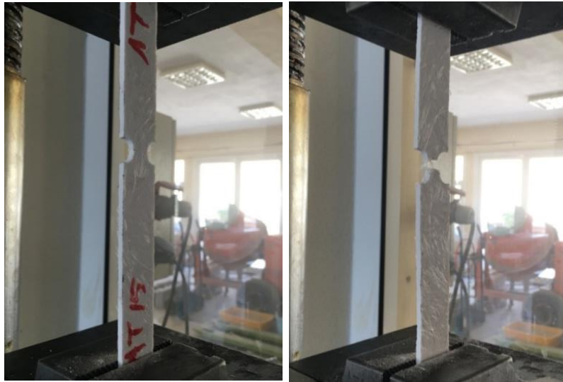
Figure 6. Condition of notched samples before tensile test and after tensile testing
