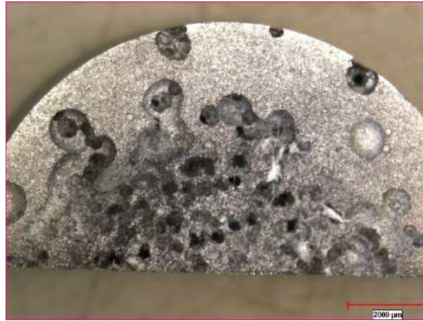
Figure 7. Image of untreated AISI 304L sample after corrosion test (at the end of the 10 th day)
