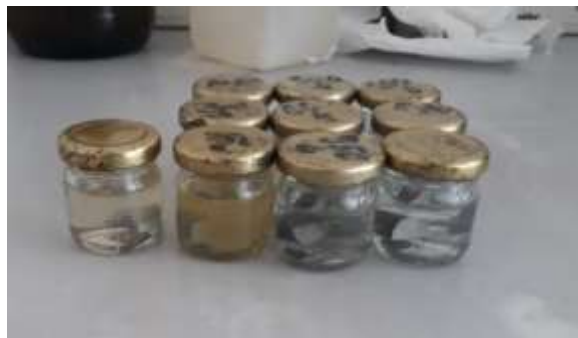
Figure 3. The samples kept in 2% \text{HNO}_3 solution
