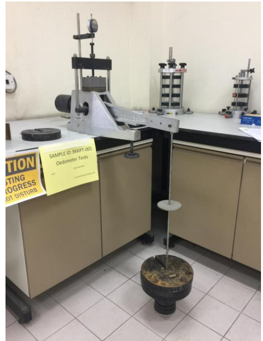
Figure 5. Laboratory testing of Klias peat soil with incremental loading of oedometer test.
