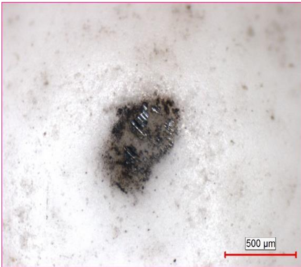
Figure 10. Wearing surface of counter element of AISI 4140 material abraded under 2N load
