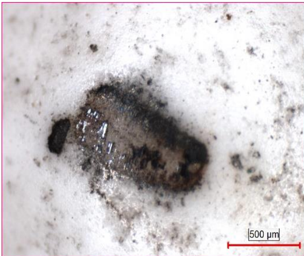
Figure 16. Wearing surface of counter element of AISI 4140 material abraded under 5N load
