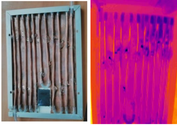
Figure 5. Backside, normal and thermal view of developed PV module
