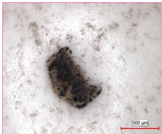
Figure 14. Wearing surface of counter element of AISI H13 material abraded under 2N load
