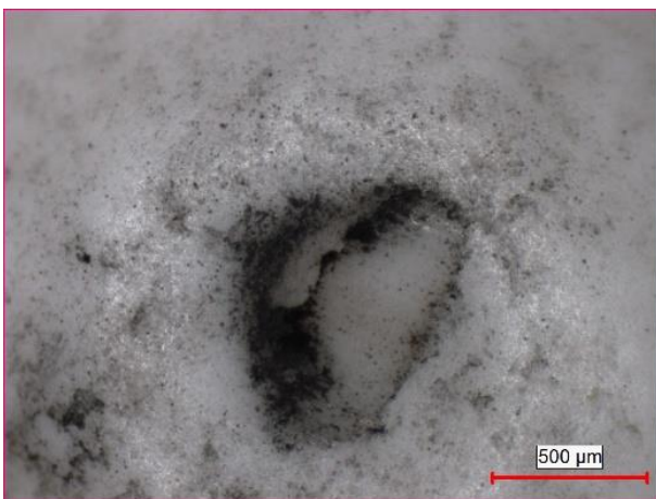
Figure 22. Wearing surface of counter element of boronized AISI H13 material abraded under 5N load
