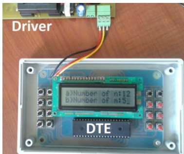
Figure. 5. Data Terminal Equipment (DTE)
