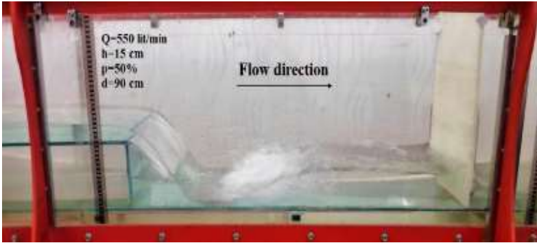
Figure 3 - Vertical drop equipped with a screen and hydraulic jump formation
